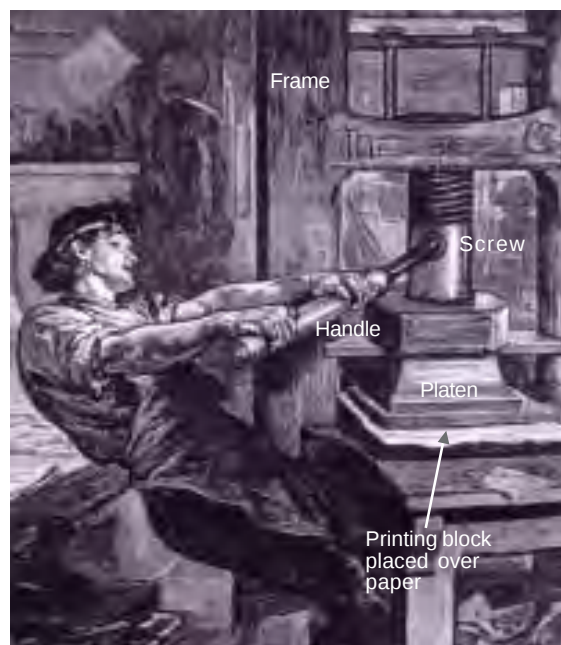
Fig. 6 – Gutenberg Printing Press. Notice the long handle attached to the screw. This handle was used to turn the screw and press down the platen over the printing block that was placed on top of a sheet of damp paper. Gutenberg developed metal types for each of the 26 characters of the Roman alphabet and devised a way of moving them around so as to compose different words of the text. This came to be known as the moveable type printing machine, and it remained the basic print technology over the next 300 years. Books could now be produced much faster than was possible when each print block was prepared by carving a piece of wood by hand. The Gutenberg press could print 250 sheets on one side per hour.
