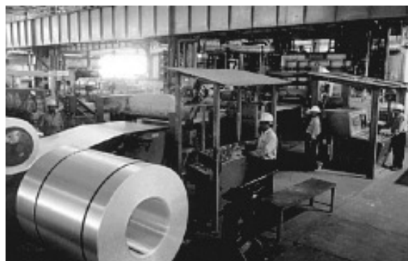
Fig. 6.6: Strip casting mill at smelter of NALCO
