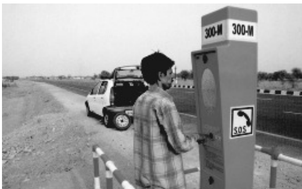
Fig.7.10 : Emergency call box on NH-8
