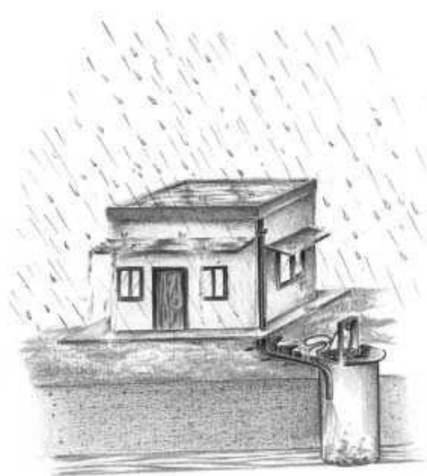
(b) Recharge through Abandoned Dugwell
