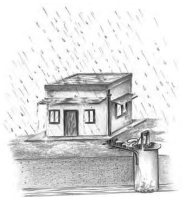
(b) Recharge through Abandoned Dugwell
